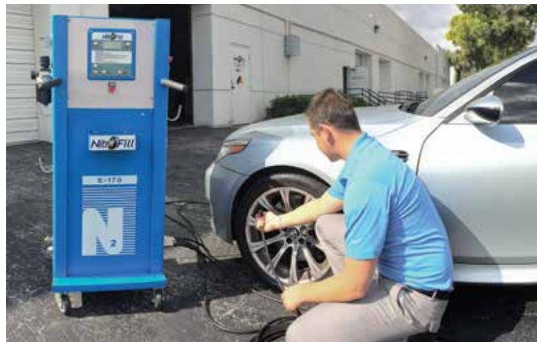
Nitrogen inflation's benefits include more stable tire pressures over the long term, less oxidation on the wheel rim for better bead sealing and longer tire life because nitrogen doesn't have the corrosive properties that come with air-filled tires.
